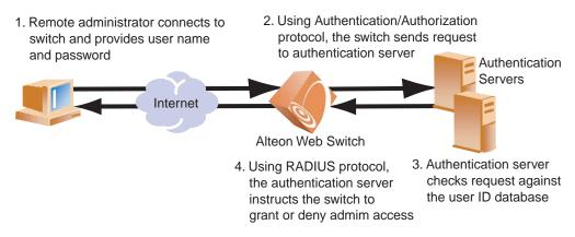
Figure 5-1 Authentication and Authorization: How It Works
